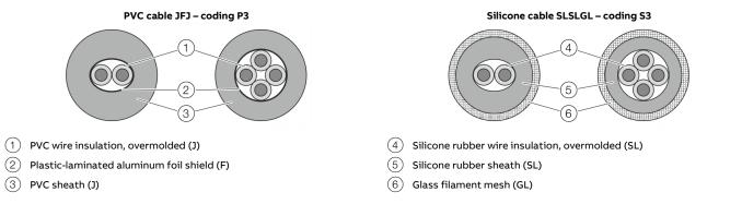
Figure 10: PVC and silicone cable
