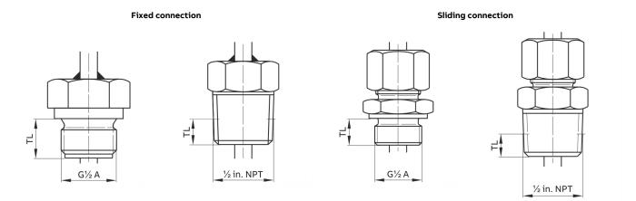
Figure 1: Screw connections types (examples)
