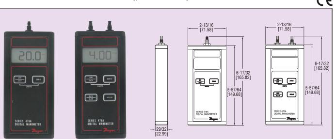
Ideal for field or laboratory use, the Model 476A Single Pressure Digital Manometer measures low pressures from -20 to 20 in w.c. with  $\pm 1.5\%$  full scale accuracy. Designed especially for the HVAC contractor, the Model 476A can be used to set supply pressures, verify pressure switch operation, adjust regulators, check pneumatic systems and computer peripherals. The rugged, handheld unit is constructed with an extruded aluminum case for exceptional durability.
