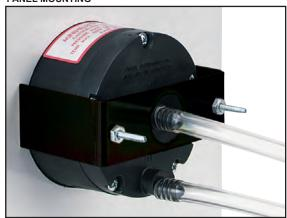
Mounting hardware is supplied with the Minihelic® II gage for panel mounting through a single hole, 2-5/8" (67 mm) in diameter. Panel thickness up to 1/2" (13 mm) can be accommodated with the hardware supplied. If necessary, surface mounting of the gage can be accomplished by means of two 4-40 screws into the tapped mounting bracket stud holes in the rear of the gage. Surface mounting requires clearance holes in the panel for the two pressure taps.
