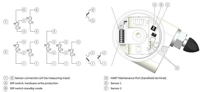
Figure 10: Electrical connections (opened connection head)
