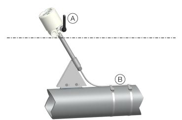
Figure 12: Temperature sensor fastening alongside the piping
