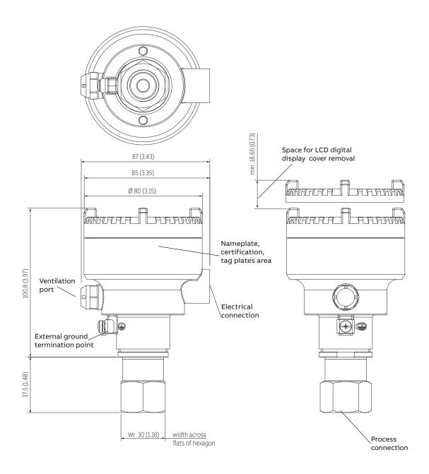
Figure 1  $\,$  PxS100 with  $\frac{1}{2}$  in NPT female connection and LCD digital display
