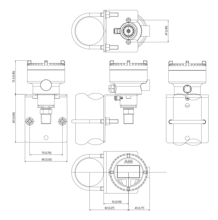
Figure 5  $\,$  PxS100 with  $\frac{1}{2}$  in NPT male /  $\frac{1}{4}$  in NPT female connection on bracket
