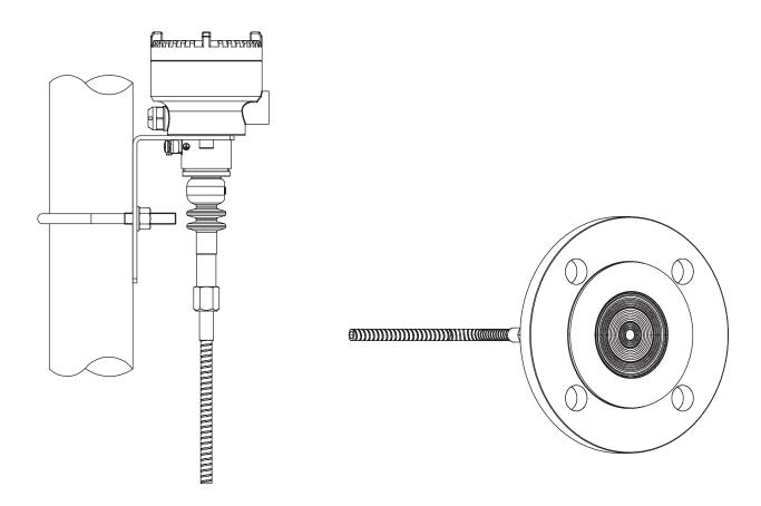
Figure 14 PxD100 with remote seal. (This is only a representative drawing. For detailed drawings of the remote seal please refer to the S26 datasheet)
