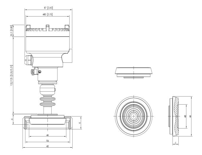
Figure 6 PXF100 with DIN11851
