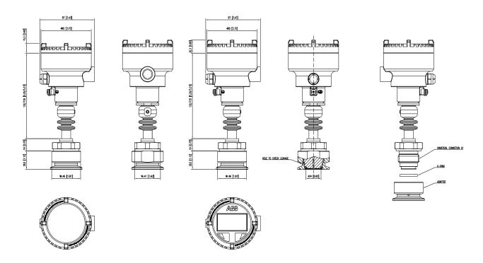
Figure 13 PXF100 with Universal connection and hygenic adapter
