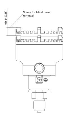
Figure 3 PxS100 with DIN-EN837-1 G 1/2 B connection
