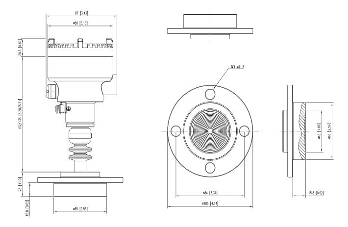
Figure 12 PXF100 with DRD
