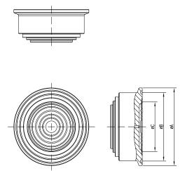
Figure 8 PXF100 with TRI CLAMP ISO 2852
