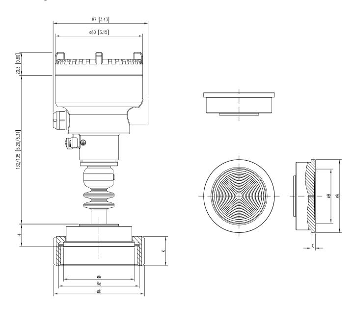
Figure 9 PXF100 with SMS SS1145
