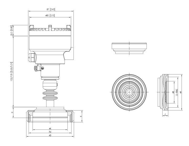
Figure 7 PXF100 with DIN11864 -1 FORM A
